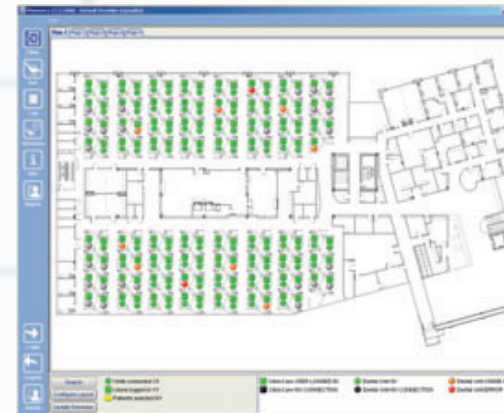
Clinic monitoring offers a graphical overview of all connected devices at the clinic. The status of each operator can be quickly evaluated and those operatories that need assistance can be immediately detected.
