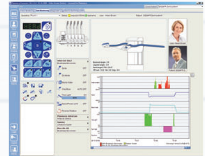
Unit view allows real-time monitoring of the selected dental unit. It can be used to monitor user activities and to review dental unit settings.
